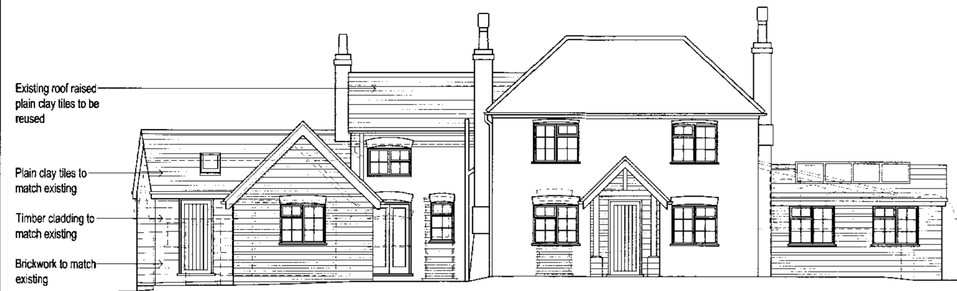
South West Elevation
